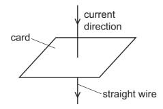
The current produces a magnetic field around the wire.
